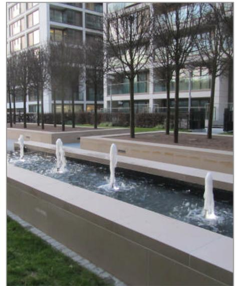
A dry mounted pumping system located within the plant room provides the supply to each jet nozzle by pumping water from a holding tank also located within the plant room. A weir edge within each raised pool allows water to fall into the two collection channels below where each drainage channel is protected by a stainless steel grille to prevent large debris from passing through and into the system.
